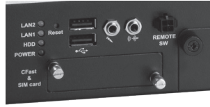
Removable CFast™, SIM slot and suspension 2.5" SATA HDD/SSD
