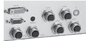
M12 connector for Giga LAN, USB 2.0 & audio port
