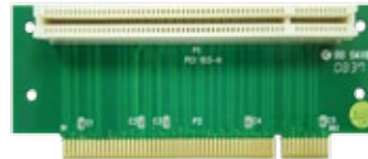
One-slot PCI riser card
