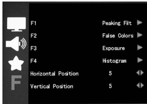
**F1:** The corresponding panel button F1 custom button function definition of choice setting(Screen marker, monochrome display, point to point, peaking focus assist, false colors filter, exposure, brightness histogram, scanning mode,center marker, segmentation).The user can enter submenu select oneitem, press the "**MENU**" is identified as the button function.
