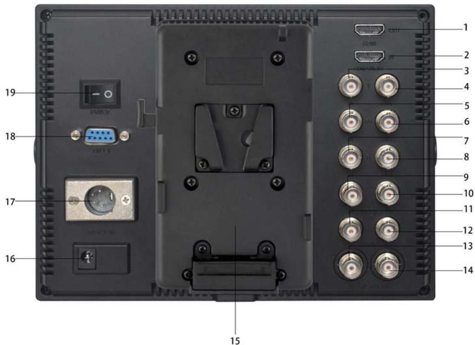
1. **HDMI OUT:** HDMI(High Definition Multimedia Interface) signal output
