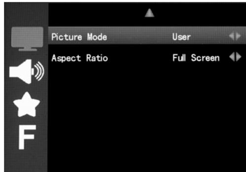
**Picture Mode:** the image brightness, standard, soft, the user (the contrast, brightness, color settings) effect settings
