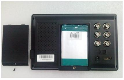
5. Lock battery cover up to finish installation.
