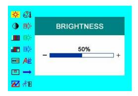
Press "</>"on the unit or " $\bigcirc$ / $\bigcirc$ " on the remote control to select item, eg.  $\stackrel{*}{\leftrightarrow}$ , and it will be highlighted; and then press +/ - of the unit or  $\bigcirc$ / $\bigcirc$  to adjust the favorite values.
