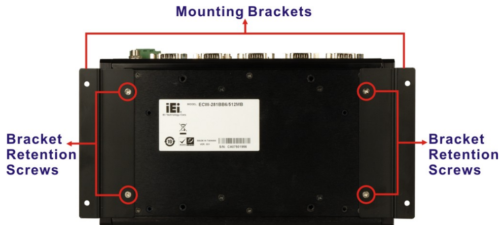
Figure 4-6: Mounting Bracket Retention Screws
