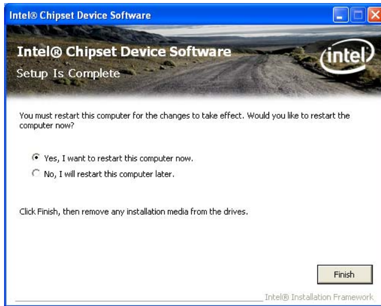
Figure 6-7: Chipset Driver Installation Finish Screen
