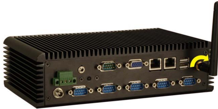
Figure 4-13: Wireless Antenna Installation
