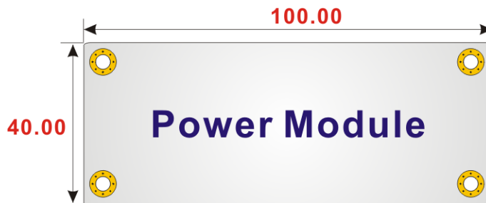
Figure 2-3: Power Module Dimensions (mm)
