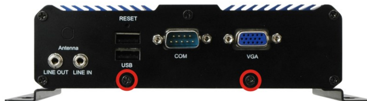
Figure 4-2: Bottom Cover Retention Screws (Rear Panel)
