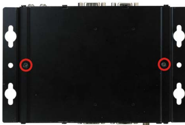
Figure 4-3: Bottom Cover Retention Screws (Bottom Panel)
