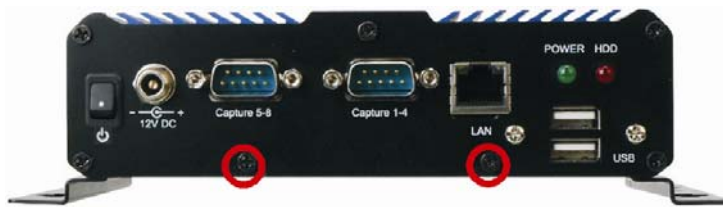
Figure 4-1: Bottom Cover Retention Screws (Front Panel)
