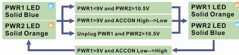
Figure 3-31: ACC On: Switch Between PWR1 and PWR2
