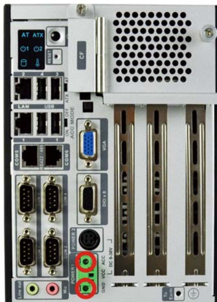
Figure 3-9: Pluggable DC-in Terminal Block Installation
