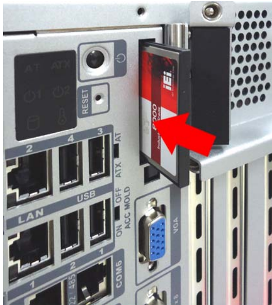
Figure 3-3: CF Card Installation
