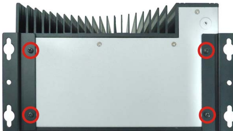
Figure 3-10: Mounting Bracket Retention Screws
