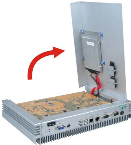
Figure 3-3: Open the Bottom Panel
