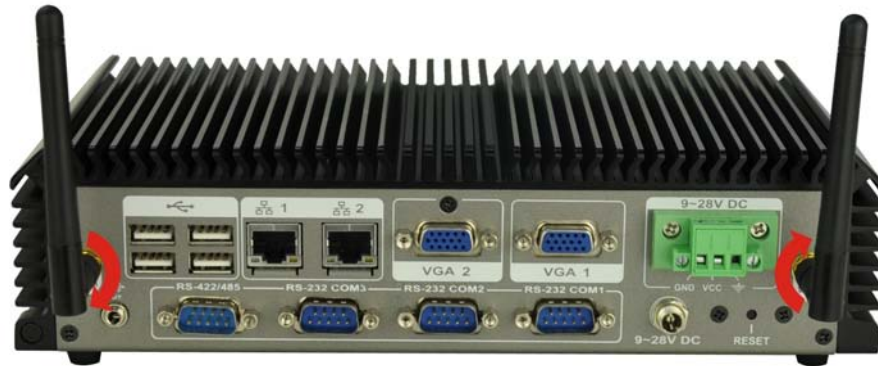
Figure 3-4: Wi-Fi Antenna Installation
