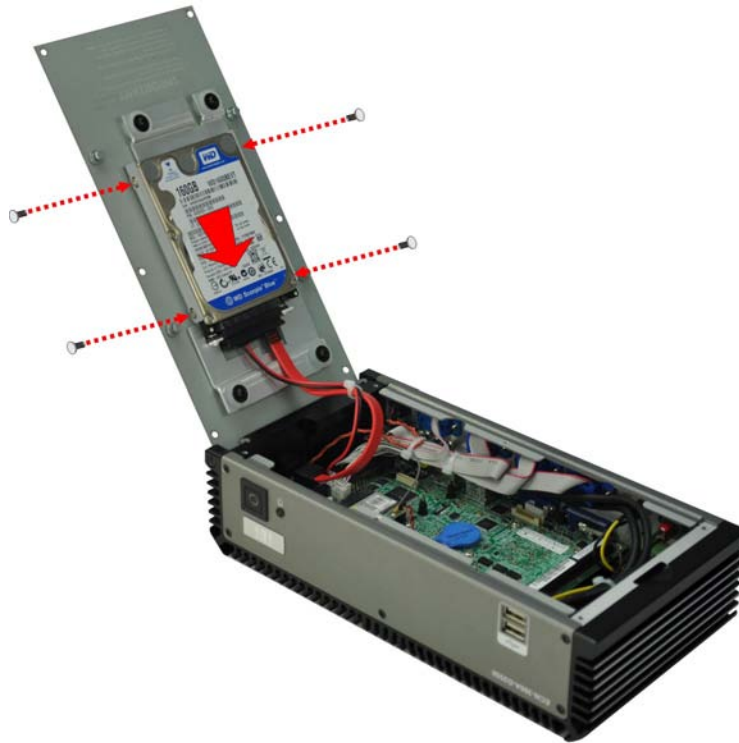
Figure 3-3: HDD Retention Screws
