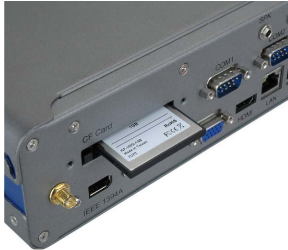
Figure 3-2: CF Card Installation
