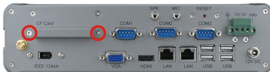
Figure 3-1: CF Card Slot Retention Screws
