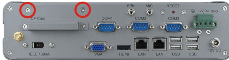
Figure 3-6: HDD Bracket Retention Screws (Rear Panel)
