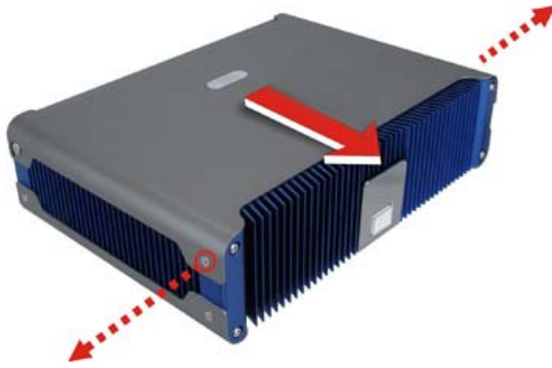
Figure 3-3: Top Panel Retention Screws Removal
