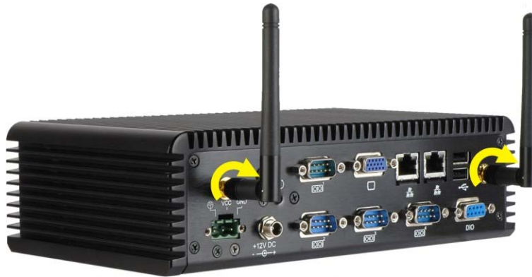
Figure 3-23: Wireless Antenna Installation
