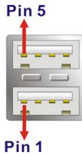
Figure 3-19: USB 2.0 Port Pinout Locations
