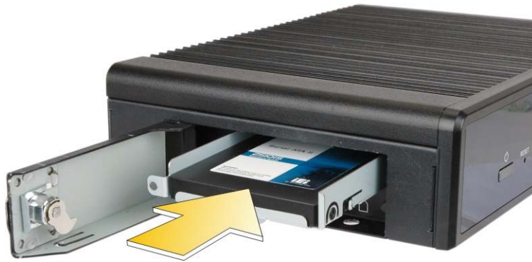
Figure 3-8: Installing the HDD
