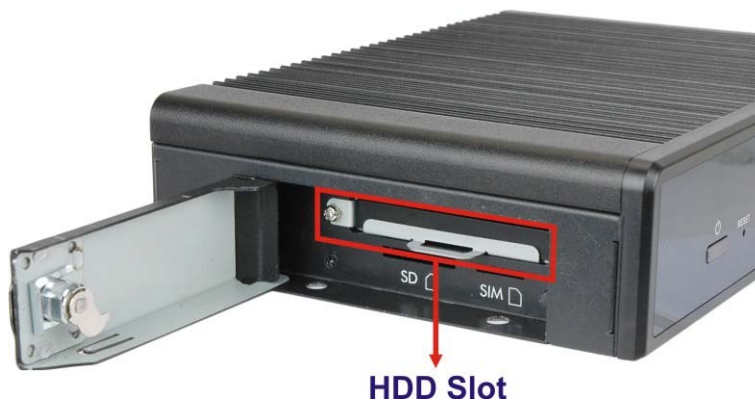
Figure 3-5: HDD Bay Location
