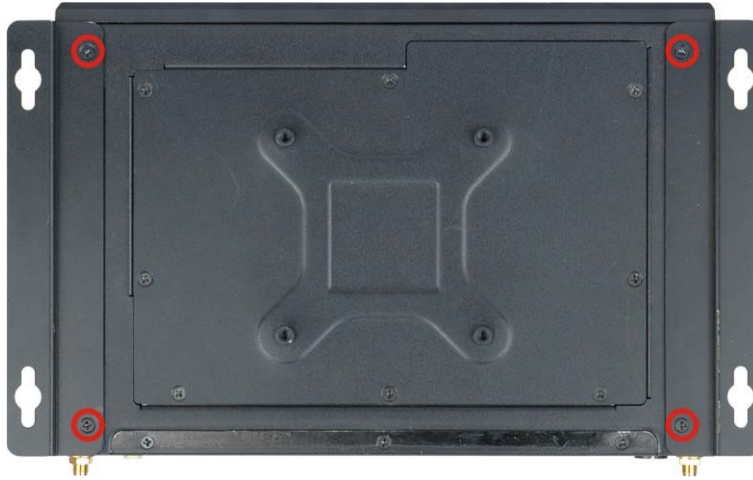
Figure 3-13: Mounting Bracket Retention Screws
