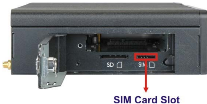
Figure 3-3: SIM Card Slot Location
