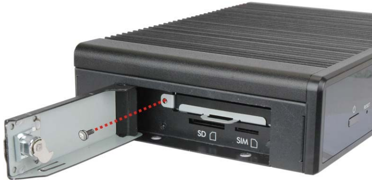
Figure 3-6: HDD Bracket Retention Screw
