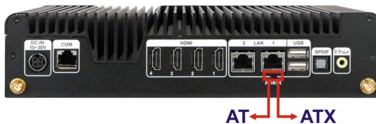
Figure 3-9: AT/ATX Switch Location
