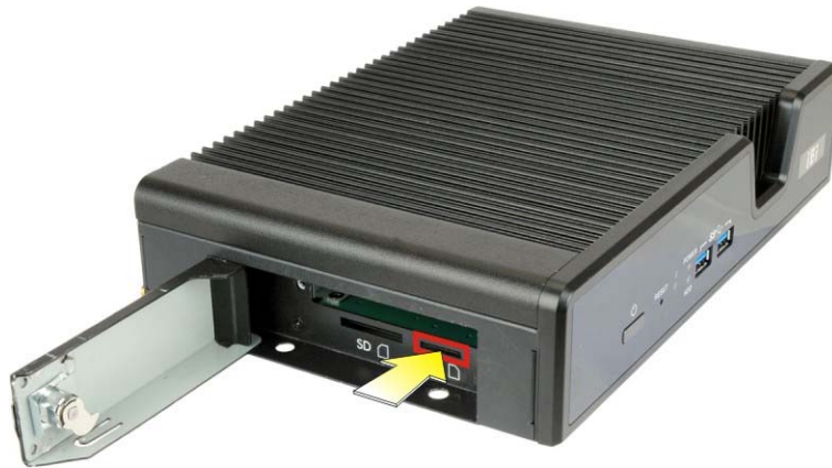
Figure 3-4: SIM Card Installation
