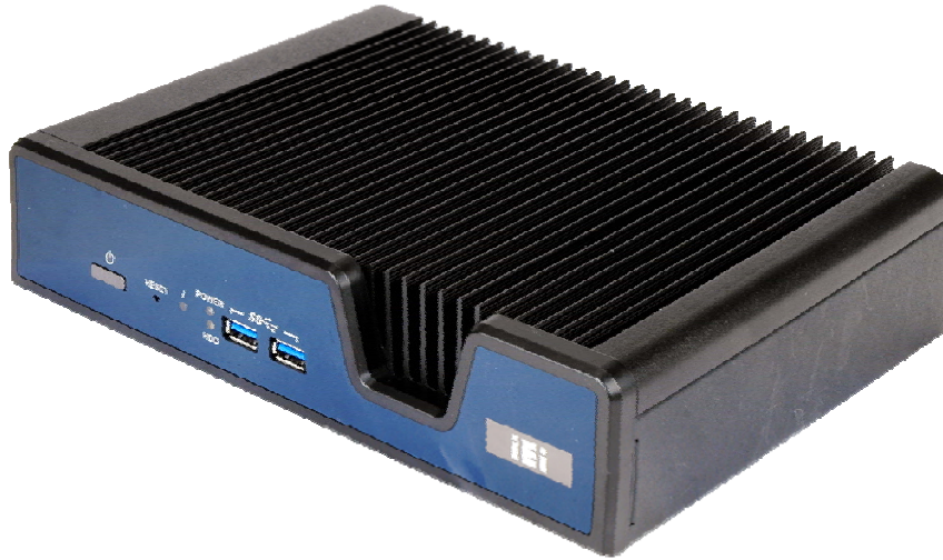
Figure 1-1: IDS-200-A70Mi Series Digital Signage Player
