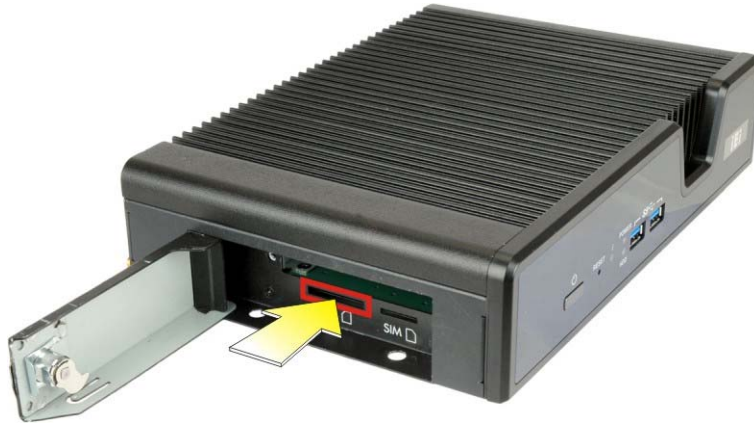
Figure 3-2: SD Card Installation
