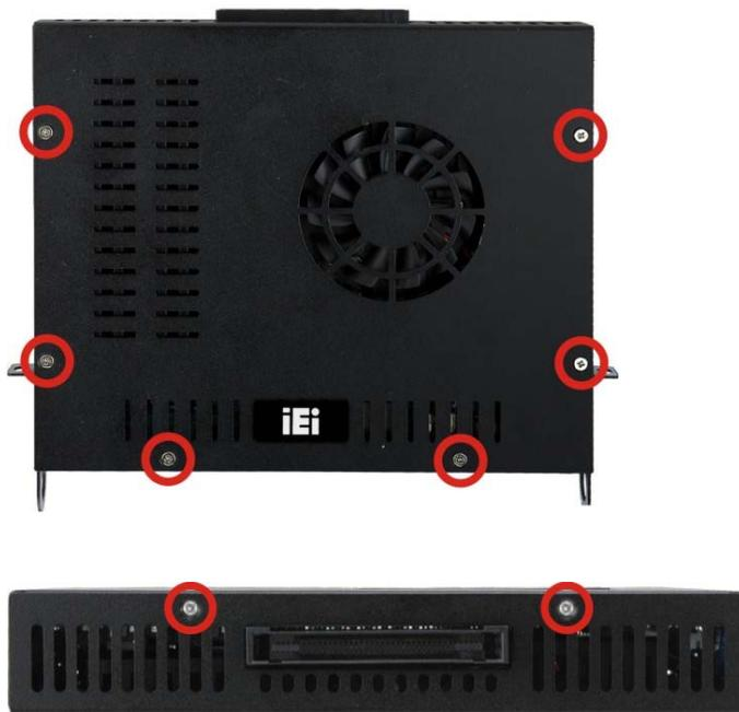
**Figure 5-1: System Cover Retention Screws**
