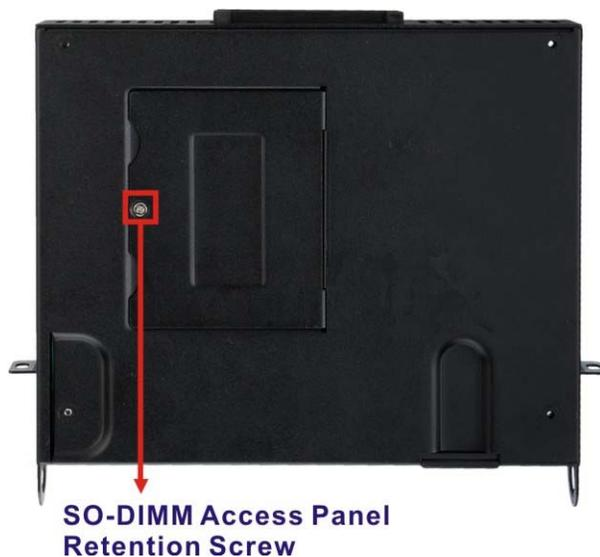
Figure 5-4: SO-DIMM Access Panel Retention Screw
