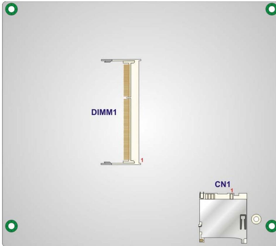
Figure 6-2: Main Board Layout Diagram (Solder Side)
