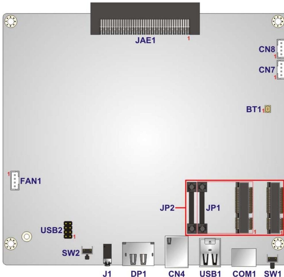
Figure 6-1: Main Board Layout Diagram (Front Side)
