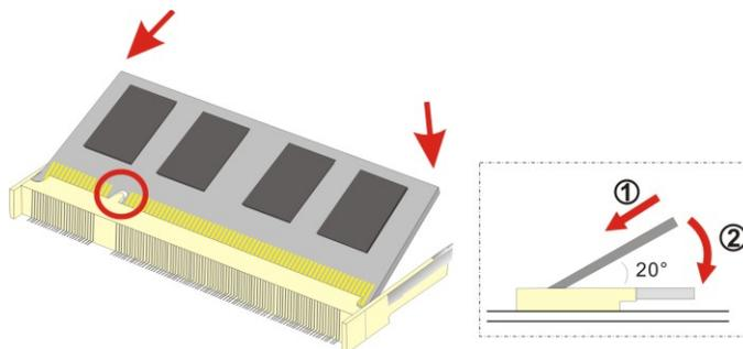
Figure 5-6: SO-DIMM Installation
