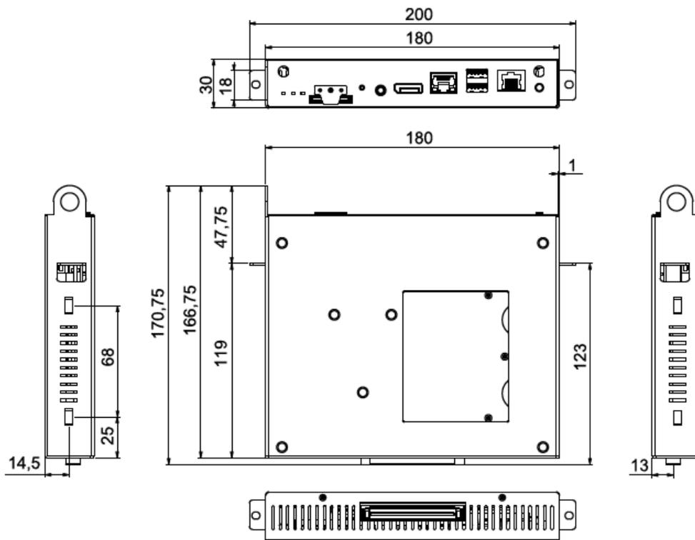
Figure 1-5: IOPS-Q67/H61 Dimensions (mm)
