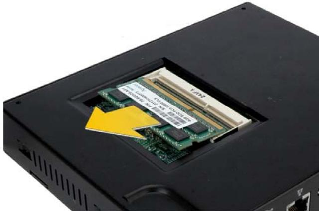
Figure 5-5: SO-DIMM Removal
