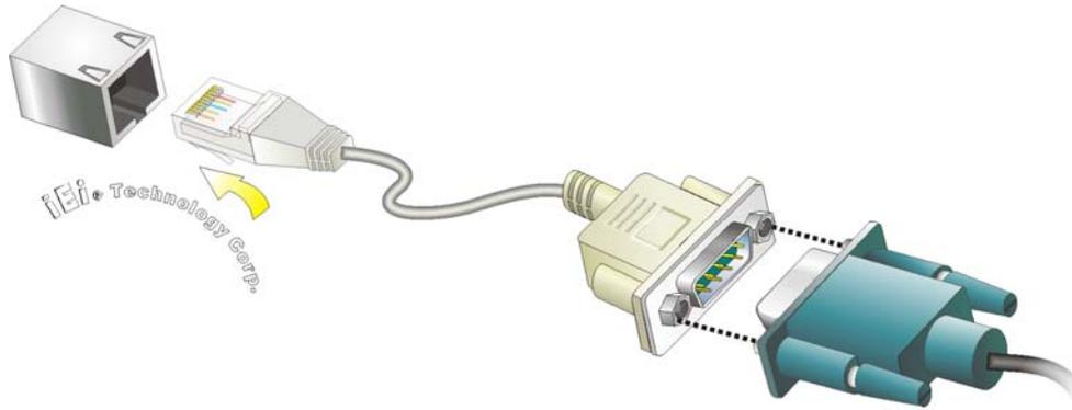
**Figure 3-6: RJ-45 Serial Port Connection**
