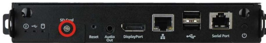
**Figure 3-1: SDHC Slot Cover Retention Screw**
