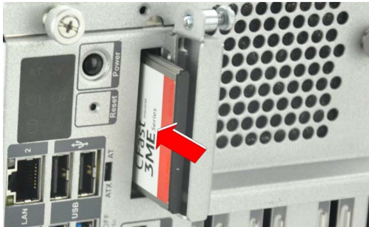
Figure 3-3: CF Card Installation
