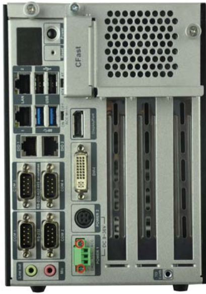
Figure 3-9: Pluggable DC-in Terminal Block Installation
