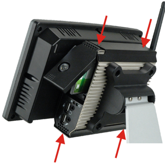
Figure 4-23: Slide Panel PC onto ulBX-200-R21/VX800
