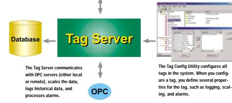
just configure which data points you want to collect and then let the Tag Server to acquire and manage the data. The Real-time Trend, Alarm Display, and User Interface controls can link to tags with a easy-to-use interface, let you view the real-time data and alarms. You can use Historical Trend to view the historical data in database. Reports control provides the data and alarm reporting function. It is so easy that you don't even need to write any program code.
