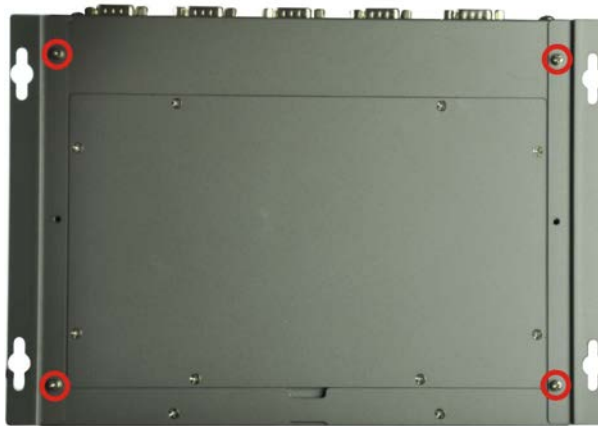
Figure 3-4: Mounting Bracket Retention Screws
