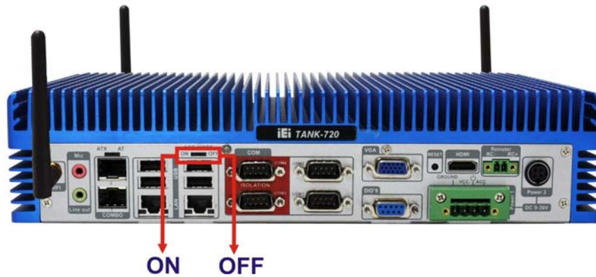
Figure 3-13: ACC Mode Switch
