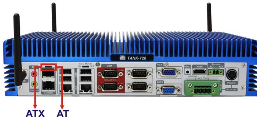
Figure 3-14: AT/ATX Power Mode Switch
