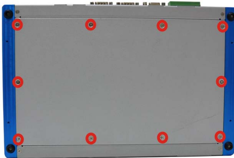
Figure 3-1: Bottom Panel Retention Screws
