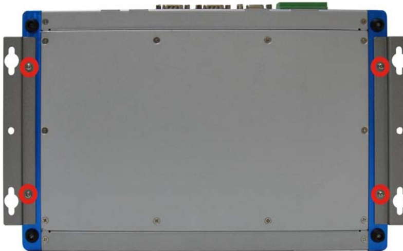
Figure 3-12: Mounting Bracket Retention Screws
