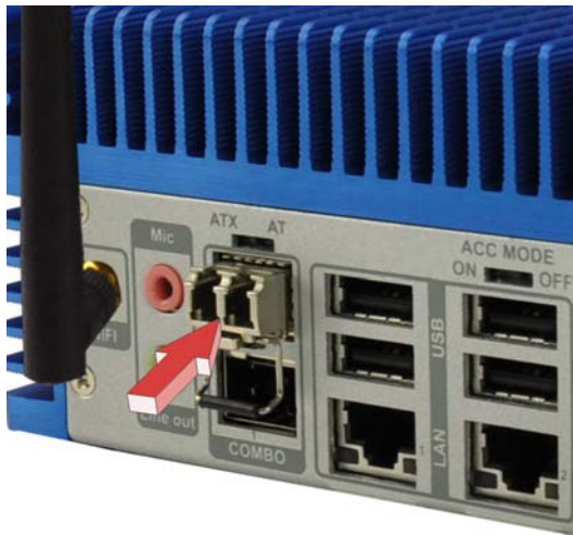
Figure 3-8: SFP Module Installation
