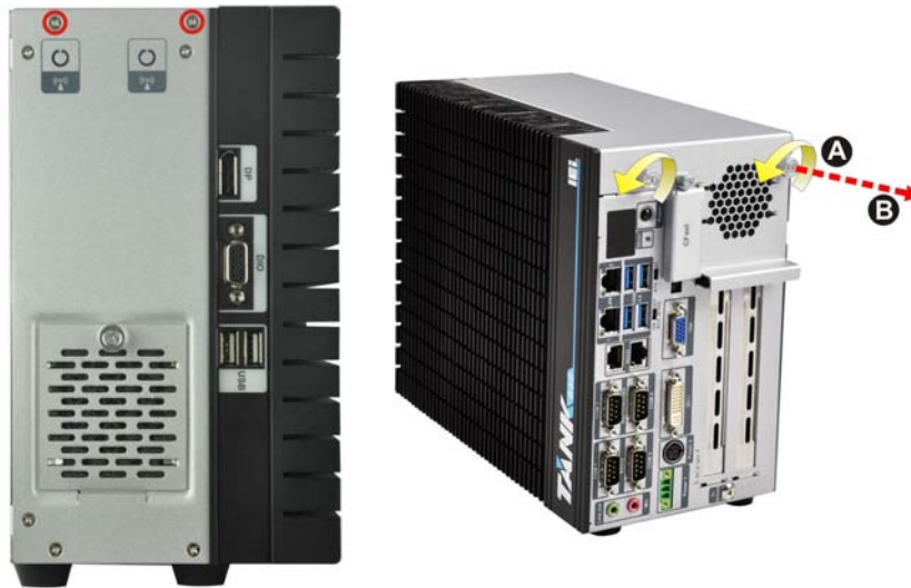
Figure 3-3: Unscrew the Cover
