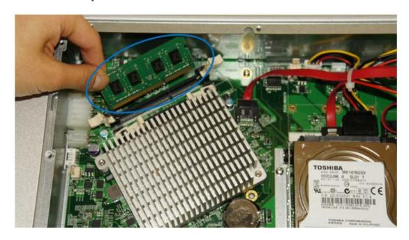
4. Place the memory module into the socket and press it firmly.
