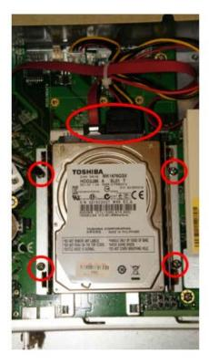
3. Remove the four screws if you want to remove and change the HDD with a different storage capacity.
