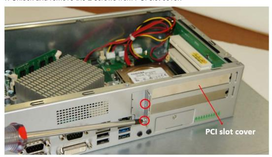
2. Remove the PCI slot cover and PCI cover bracket from inside.
